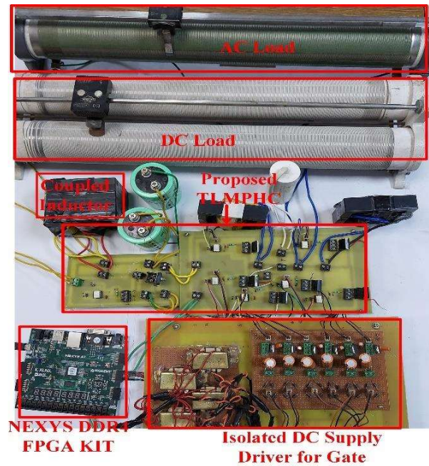
Fig. 3.11 Photograph of the experimental set-up of TLMPHC
