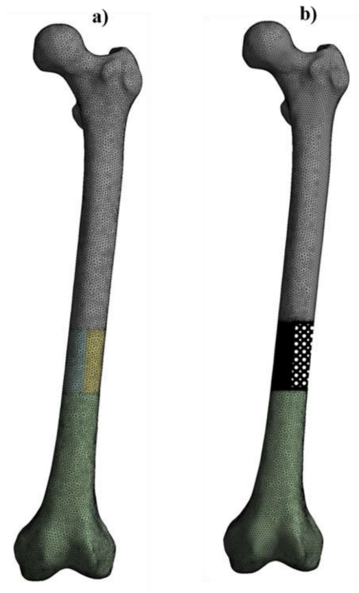
Figure 7.18: Illustration of mesh generation a) Femur with solid scaffold a) Femur with anatomically matched P scaffold.
