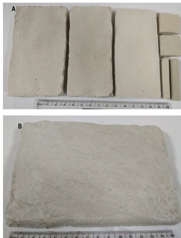
Fig. 2 – Image of (a) different size CSB samples and (b) pilot size sample.
