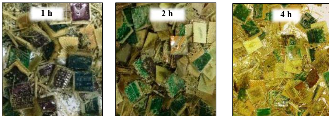
Figure 3.28- Dissolution of solder mask after different time [WPCB:DMA- 3:10, 160 °C, WPCB size- 1 cm 2 ]
