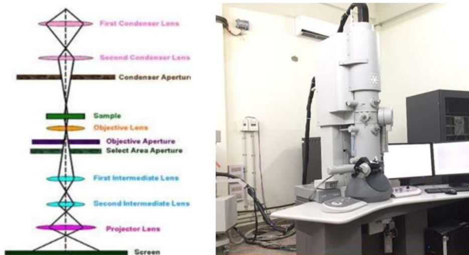
Figure. 4.9 Schematic representation of the principles of transmission electron microscopy (TEM) and a photograph of a TEM.
