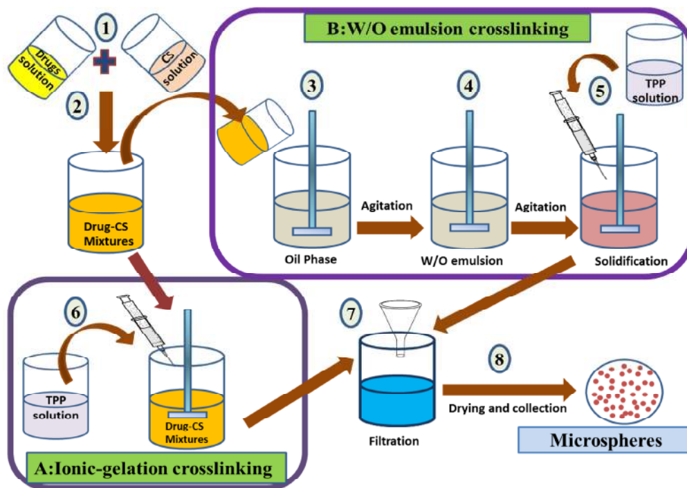
Figure 5.2: Diagrammatic illustration of ionic-gelation crosslinking (Method A) and w/o emulsion crosslinking method (Method B) for preparation of microspheres. ① Dissolution of drugs and polymers in respective solvents (Method A and B); ② Mixing of drug solution and polymer (Method A and B); ③ Dropping of drug-polymer solution to liquid paraffin (Method B); ④ Formation of stable w/o emulsion (Method B); ⑤ Dropping of crosslinking agent to solidify the formed aqueous droplets in w/o emulsion with the help of syringe (Method B); ⑥ Addition of crosslinking agent directly to the drug-polymer solution (Method A); ⑦ Filtration and washing (Method A and B); ⑧ Drying and collection of microspheres (Method A and B).
