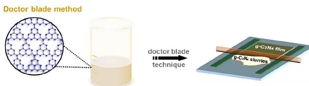
Figure 1.9: Doctor Blade method for coating of gCN slurry. Permission taken from ref[90].
