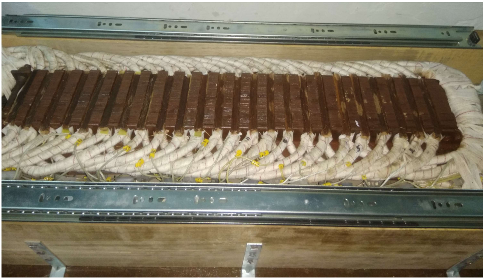
Fig. 3.9 Prototype SLIM stator with sliding support for secondary sheet
