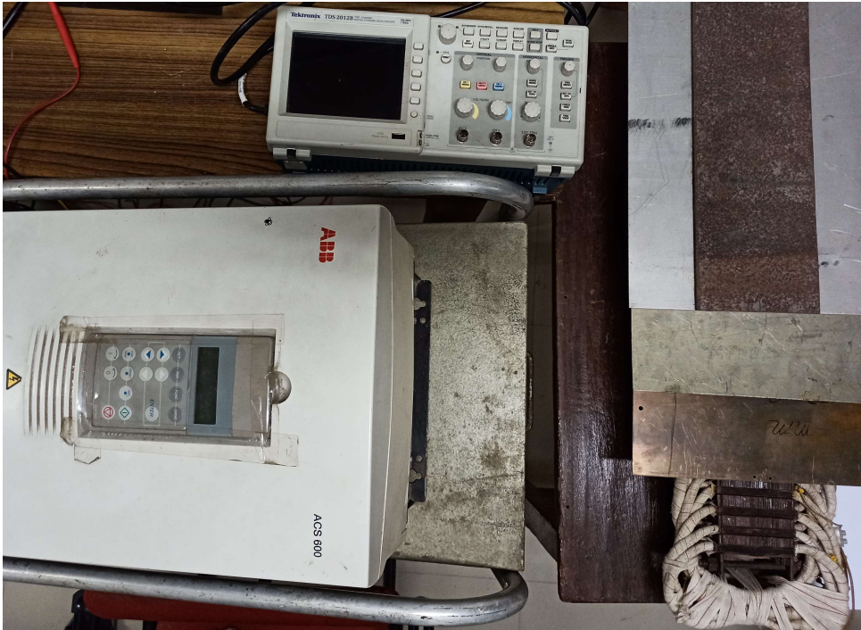
Fig. 3.10 Setup for testing of the prototype SLIM
