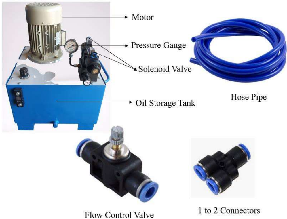
Figure 3.7: Hydraulic power pack main components
