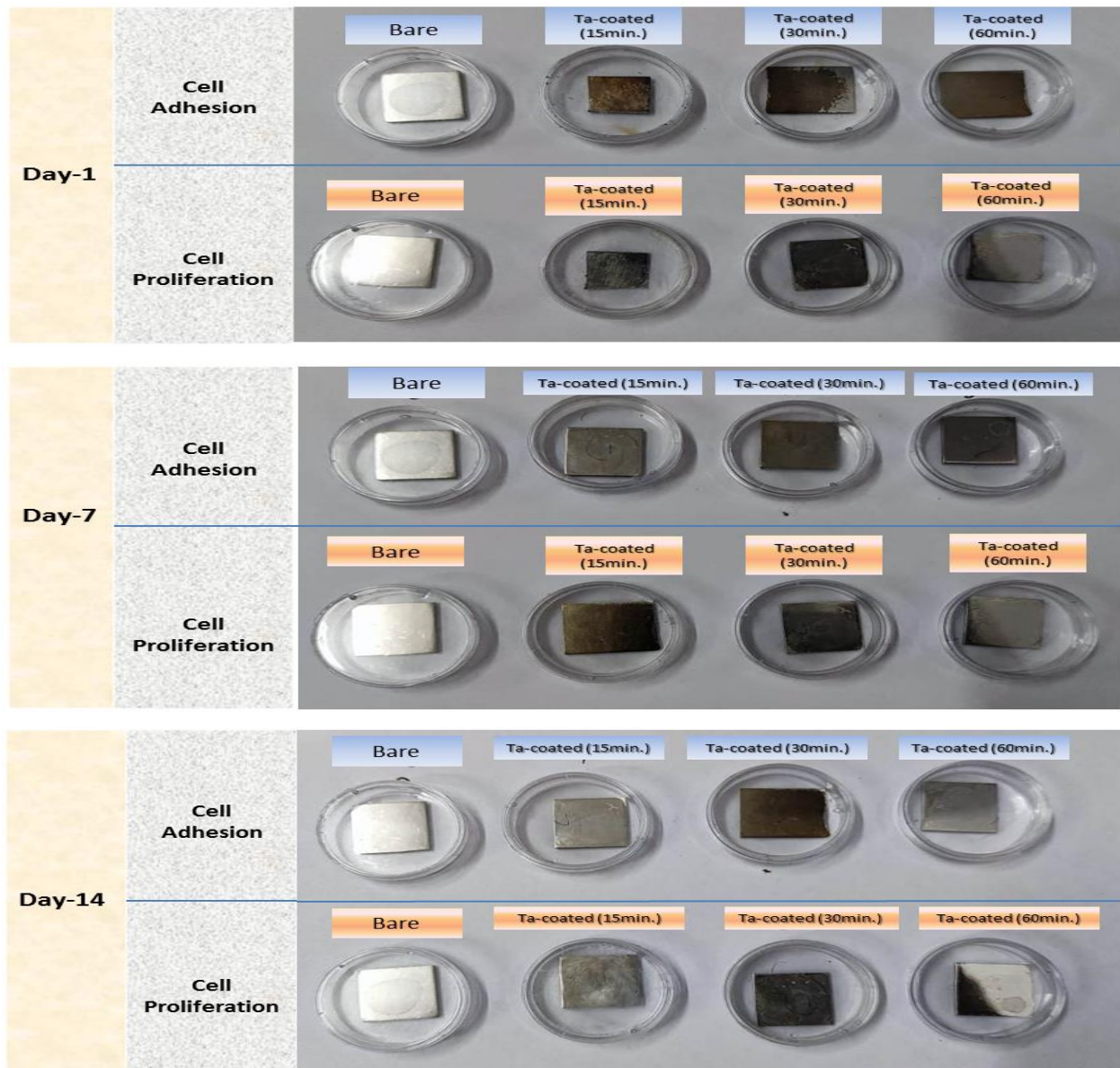
Fig. 6.12 Photographic images of bare and Ta-coated 316L SS for biocompatibility test
