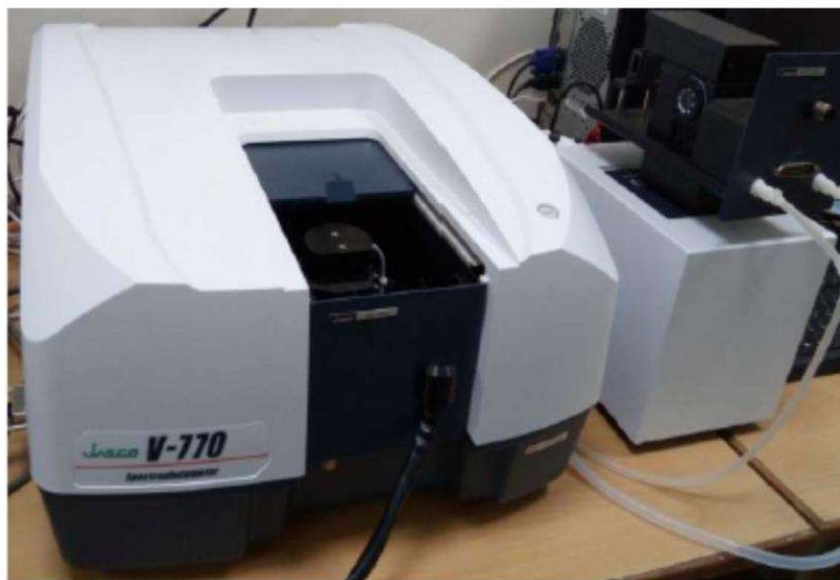
Figure 2.7: UV-Visible spectrometer set up.
