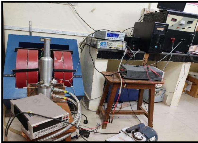
Figure 2.5: Dielectric and magneto-dielectric measurement setup.
