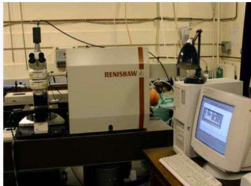
Figure 2.6: (a) Illustration of Raman effect using energy level diagram 64 . (b) Display the picture of the Renishaw micro-Raman spectroscope used in our characterization.
