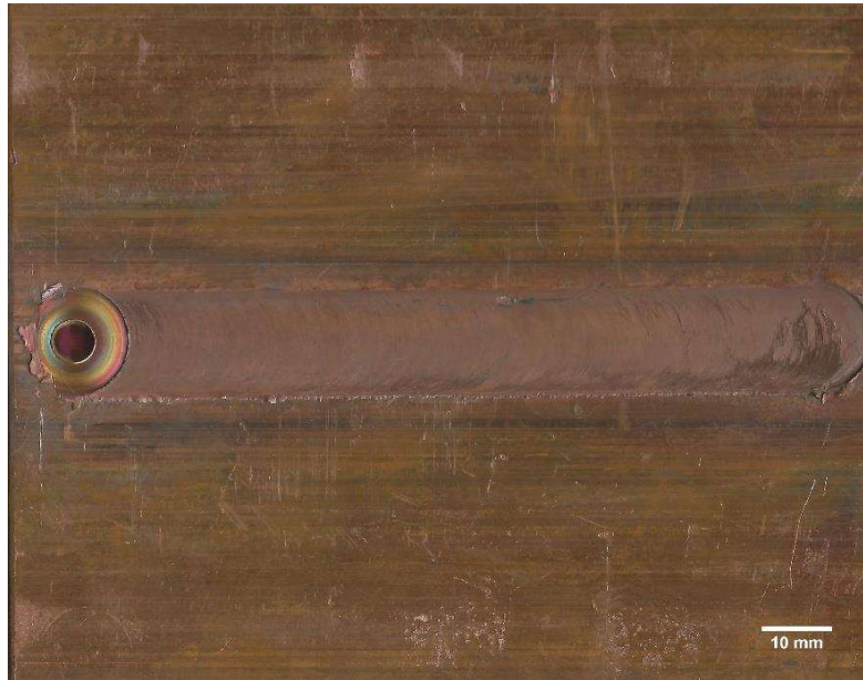
Figure 4. 1 Surface appearance of FSPed Cu/ZrSiO 4 surface composite
