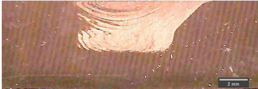
Figure 4. 2 Cross-sectional macrostructure of FSPed Cu/ZrSiO 4 surface composite
