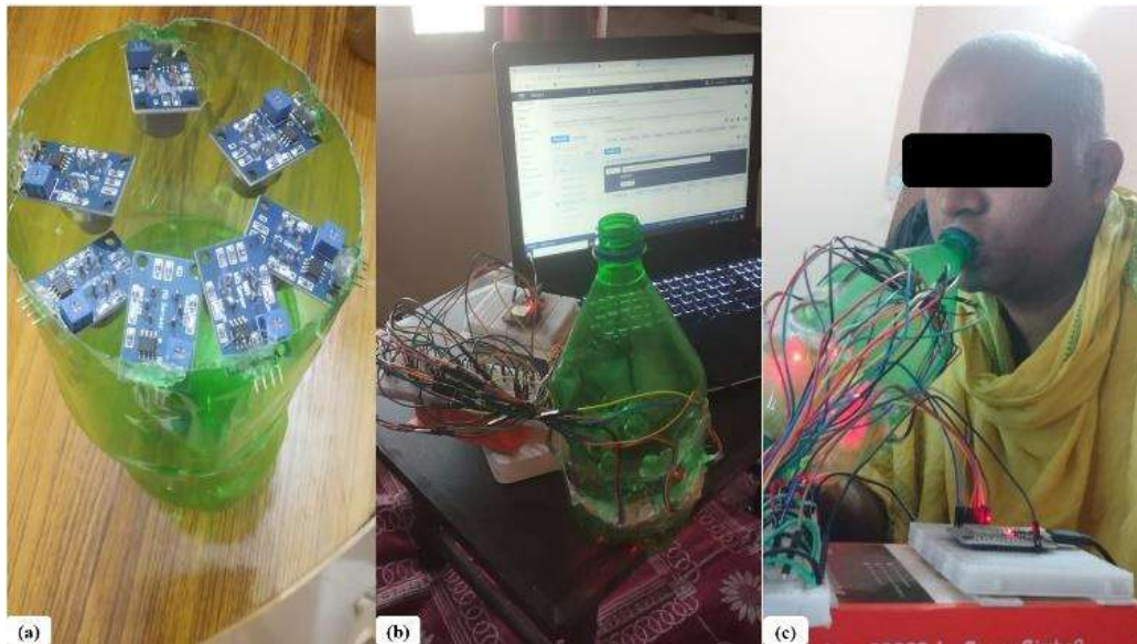
Figure 7.5 (a) Placement of sensors, (b) Sensor node connection with cloud, and (c) Physical test procedure.
