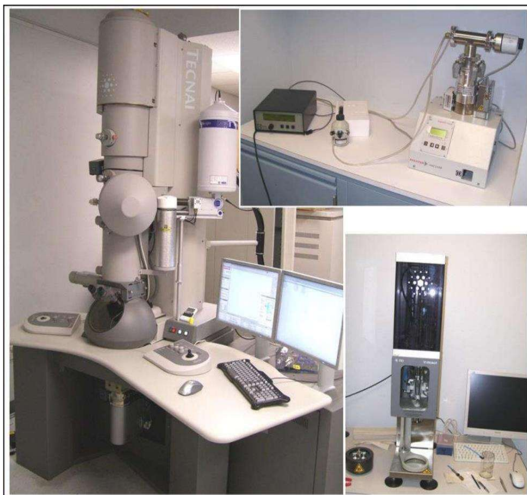
Figure 2.5. Transmission Electron Microscope (TEM, FEI TECANI G 2 20 TWIN, USA) used to determine particle structure.
