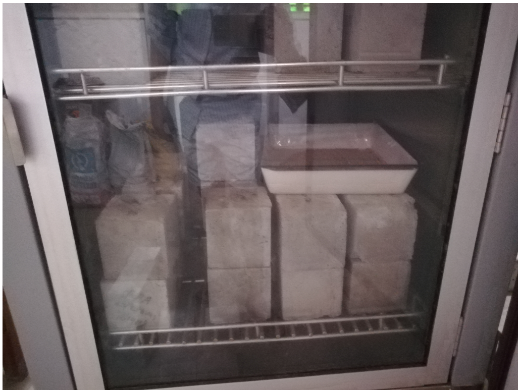
Figure 3.16: Accelerated carbonation curing
