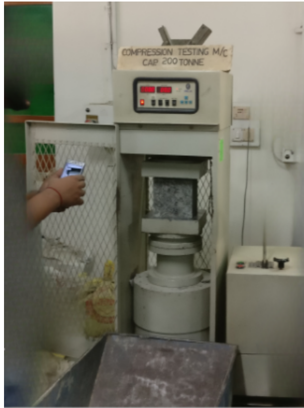
Figure 3.10: Compressive strength testing arrangement
