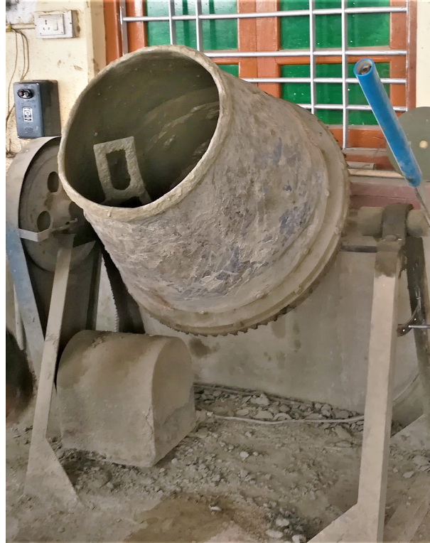
Figure 3.7: Concrete drum mixer
