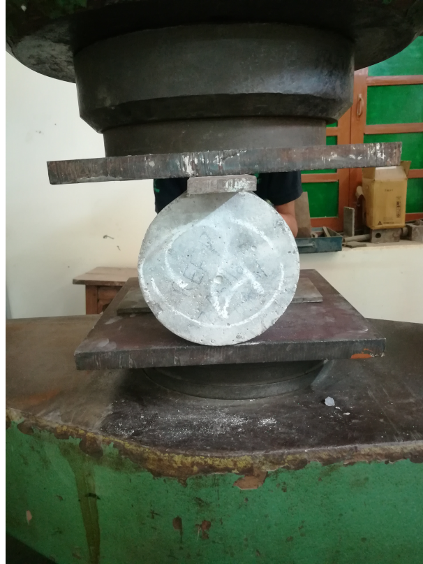
Figure 3.13: Splitting tensile strength testing arrangement
