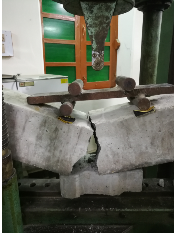
Figure 3.14: Flexural strength testing arrangement
