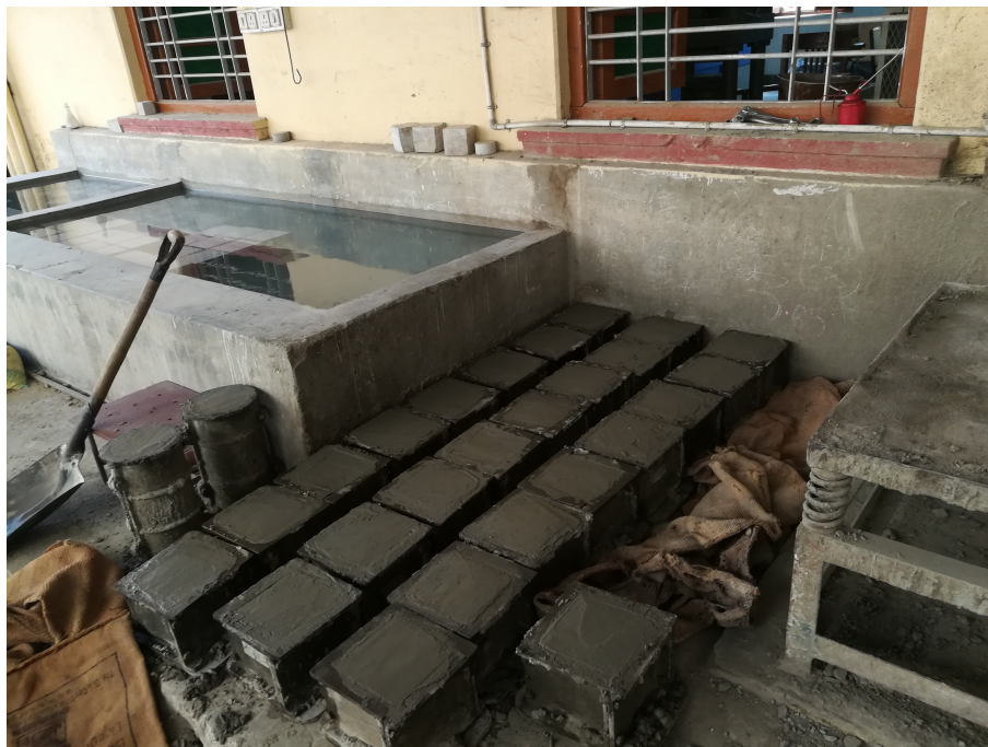
Figure 3.11: Cube casting for Compressive strength testing
