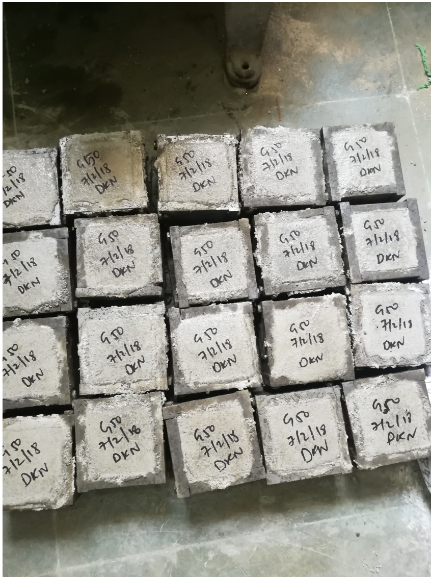
Figure 3.5: Casting of 100 mm cubes
