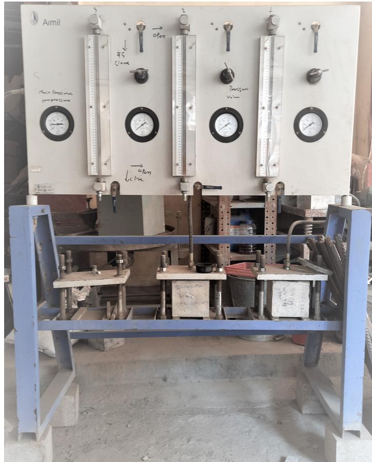
Figure 3.15: Water permeability testing arrangement
