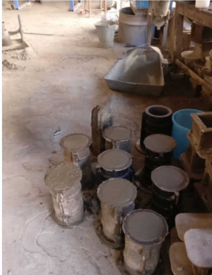
Figure 3.12: Cylinder casting for splitting tensile strength test
