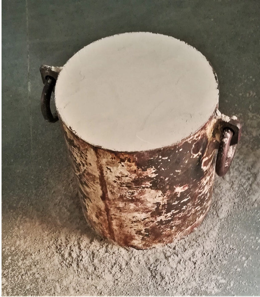
Figure 3.4: Cylinder for unit weight calculation
