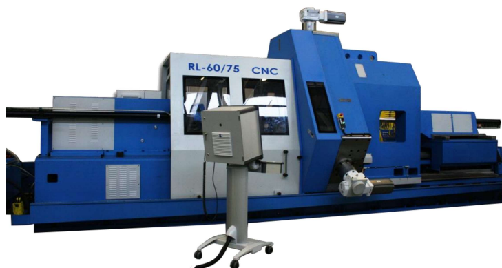
Figure 1.4: A typical flow forming machine [8]
