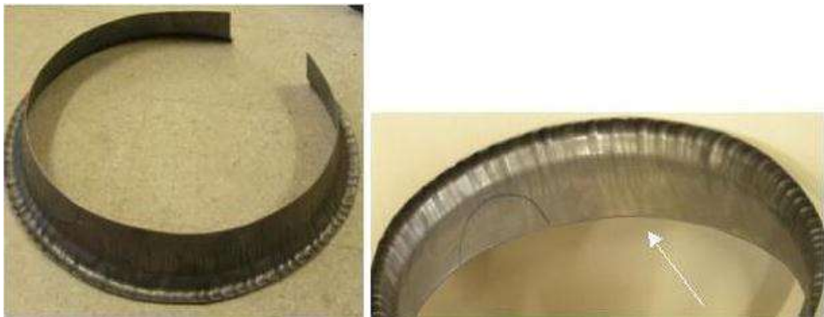
Figure 1.13: Wrinkling defect Gupta et al. [23]
