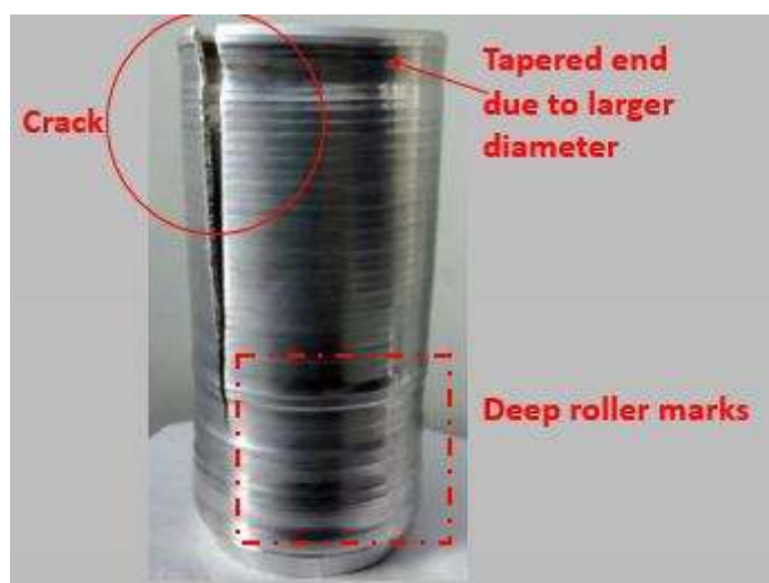
Figure 4.60: Defects in flow formed Al2014 product.
