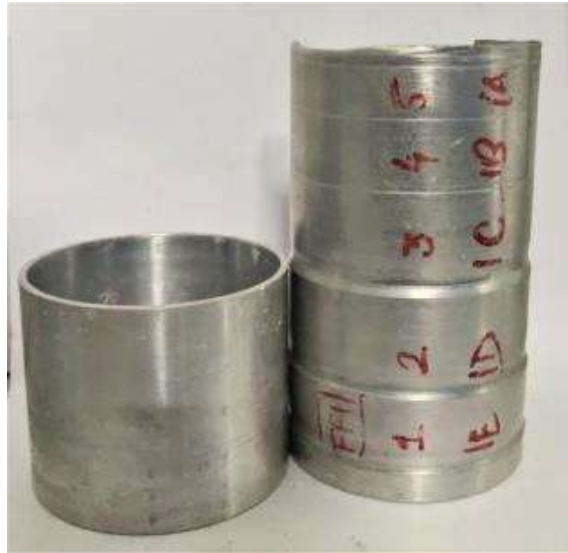
Figure 4.2: The preform and the flow formed product showing the different regions. IE represents the initial region (not flow formed) while regions 1A-1D denote the thickness reduction obtained in 4 different passes
