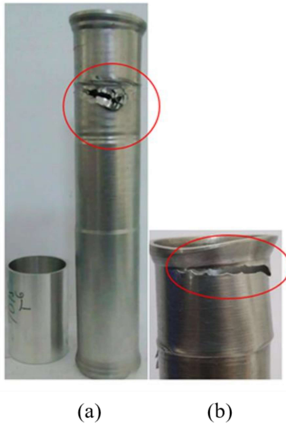
Figure 4.43: Flow formed 7F05 (a) preform and flow formed product (b) crack near the end and ovality at end section.
