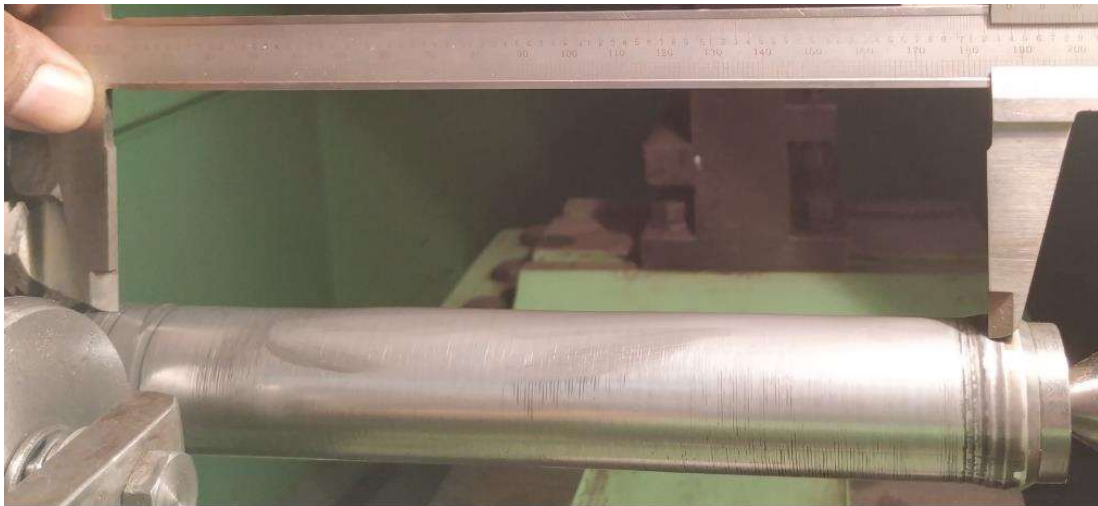
Figure 4.23 Flow formed Al7075 annealed sample 7F04
