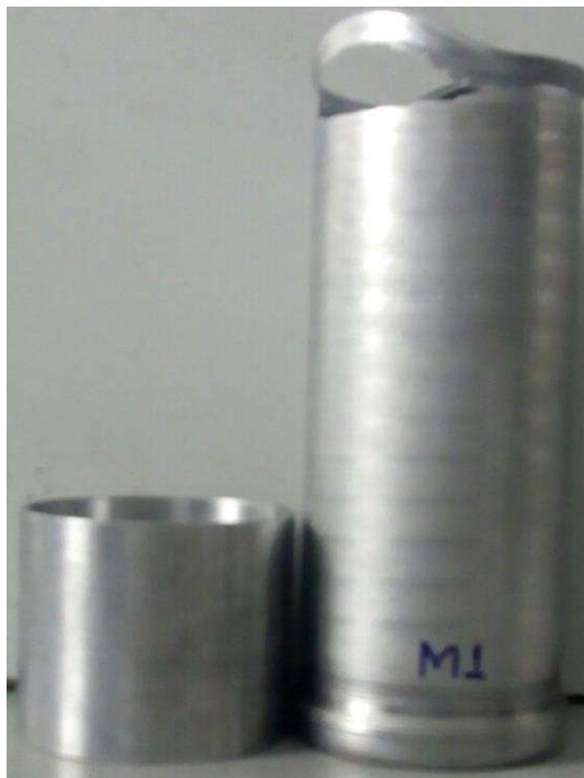
Figure 4.8: Preform and Flow formed FF03
