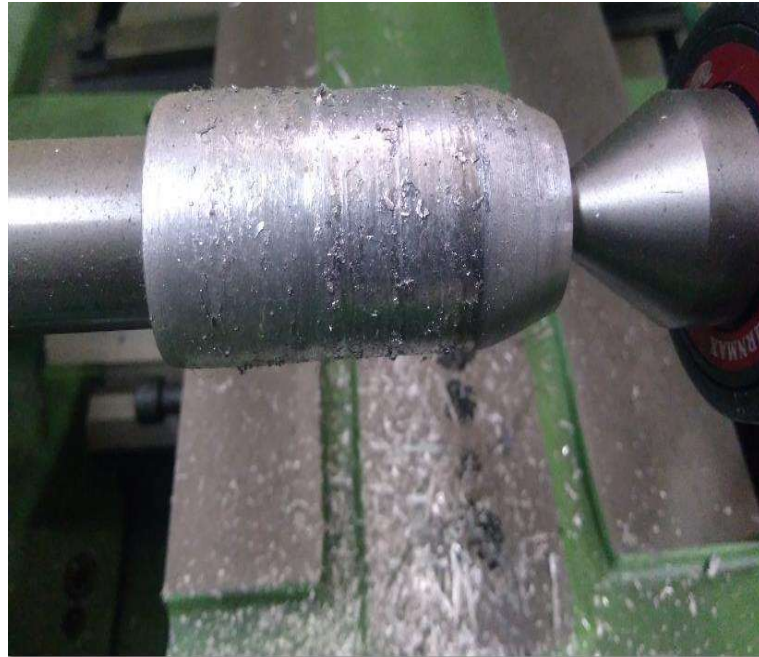
Figure 4.37: Defect: Chip formation during flow formation.
