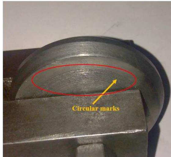
Figure 4.38: Defect: Circular marks in Roller
