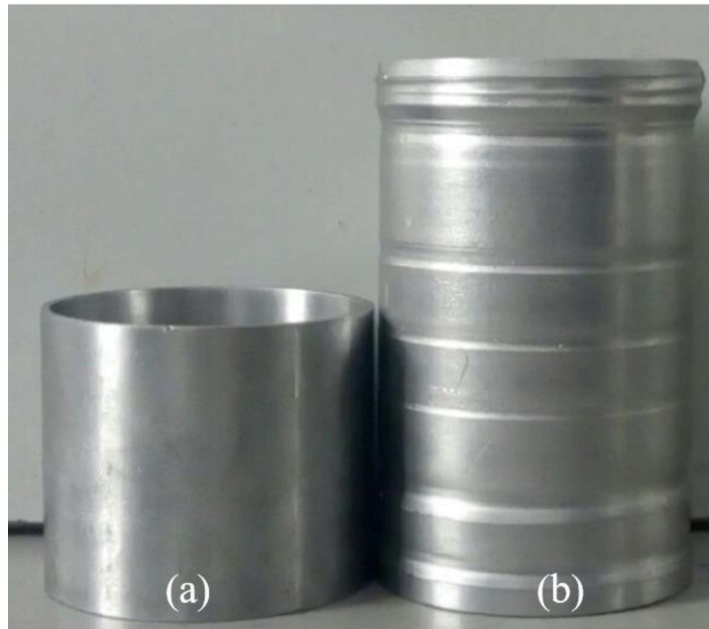
Figure 4.7: Flow formed FF02-Multistep flow formed sample (a) preform (b) Flow formed product.
