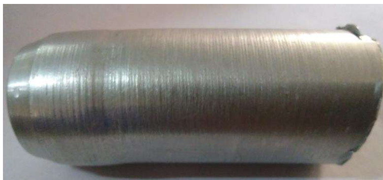
Figure 4.39: Bending of Job Flow formed Aluminium 6061(as received) with Roller attack angle of 30^\circ . Rotation speed of 420 RPM.
