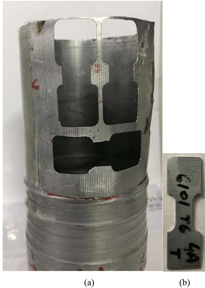
Figure 4.12: (a) Tensile specimen cut out from flow formed FF04. (b) One Tensile specimen
