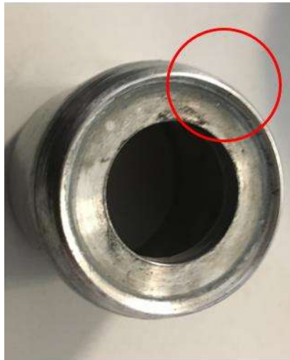
Figure 4.36: Backward flow defect leading to flange formation
