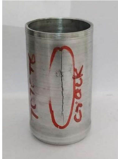
Figure 4.21: Flow formed 7F02 showing crack formation in the middle of the specimen.
