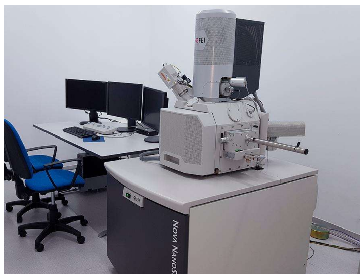
Fig. 2.4 HR-SEM and EDS set up.
