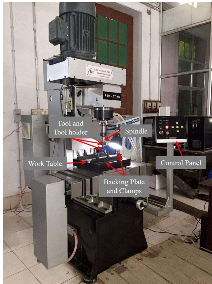
Figure 3. 4 Friction stir processing set-up
