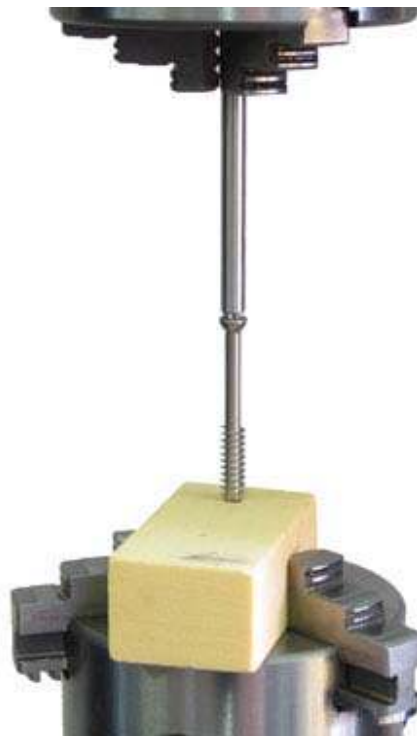
Figure 1.30: Schematic illustration of pullout test for metallic medical bone screws.
