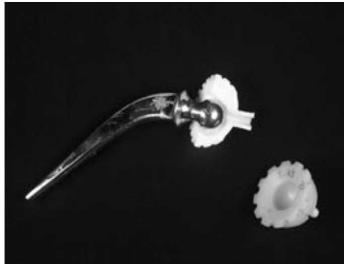
Figure 1.24: Charnley low-friction THR with small stem and ultra-high molecular weight polyethylene (UHMWPE) socket from 1962. Picture from (Reynolds et al., 2007)
