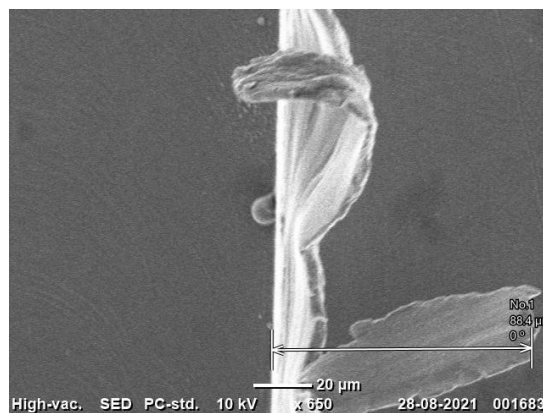
Fig. 6.9 Typical SEM image denoting burr width measurement in down milling
