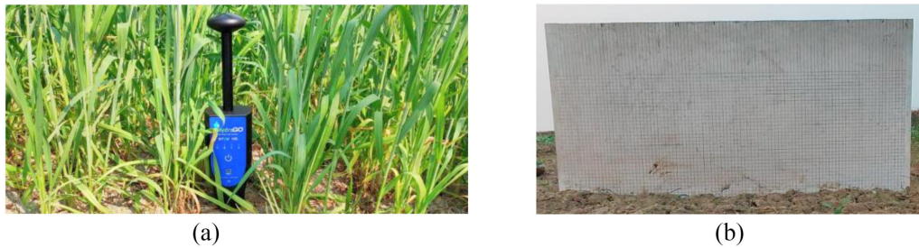
Figure 4.2 The procedure of measuring (a) soil moisture using HydraGO, (b) surface roughness profile.
