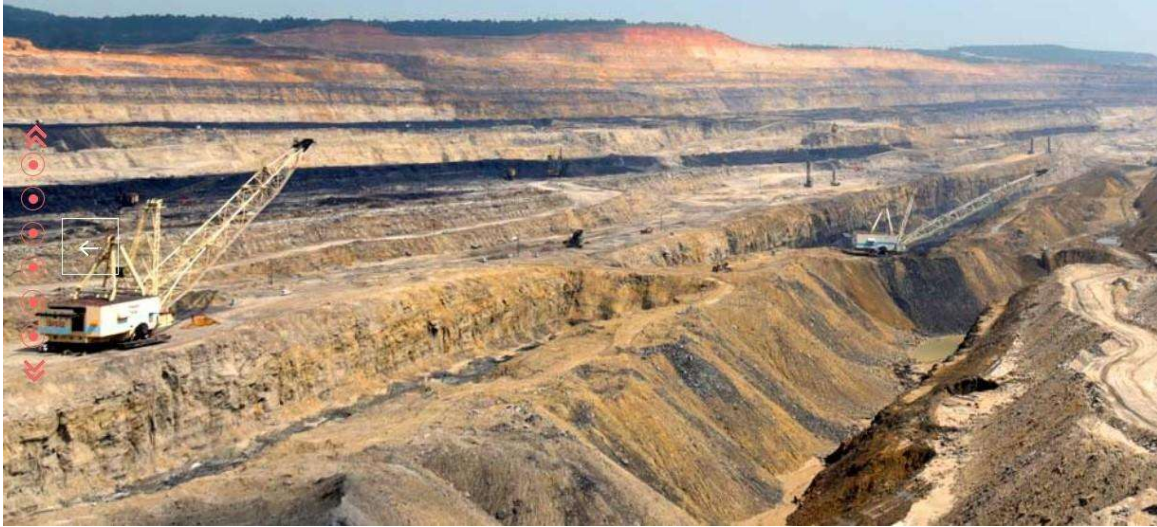
Figure 2.14: Two draglines working in vertical tandem at Bina mine of NCL.
