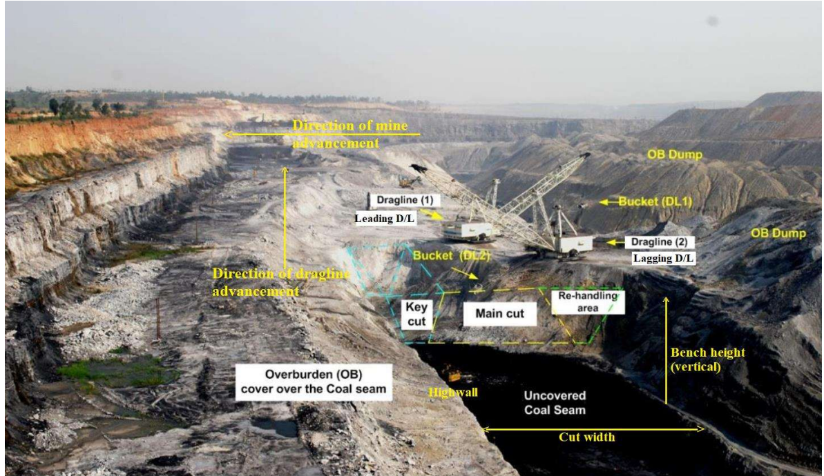
Figure 2.11: Two draglines working in horizontal tandem with key terms elaborated. (Modified from Mousa and Rai,2015)
