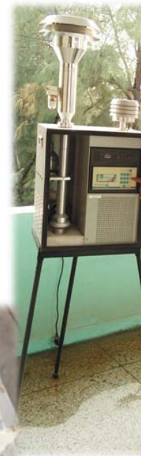
d) Ambient fine dust sampler (Model Instrument IPM–FDS 2.5/10 \mu )
