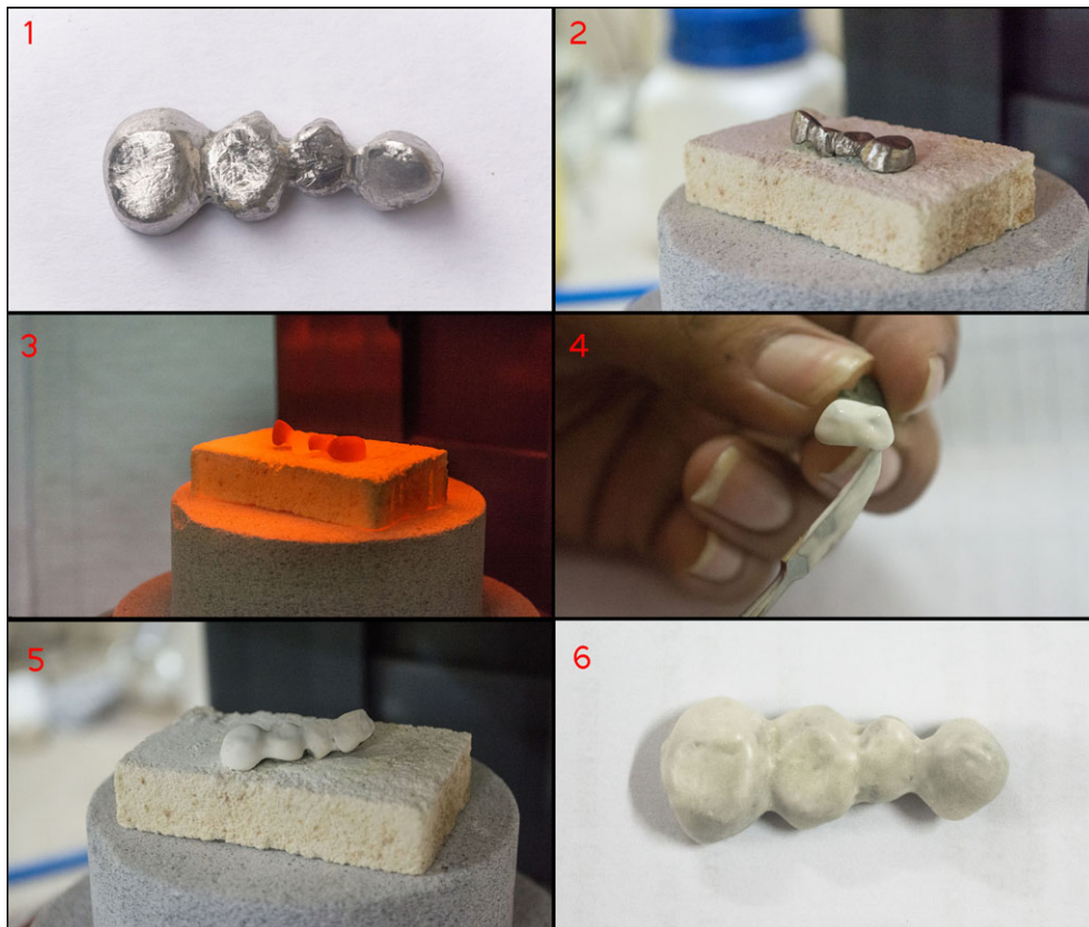
Fig. 5. Kalsilite glass-ceramic opaque material applied on metal.
