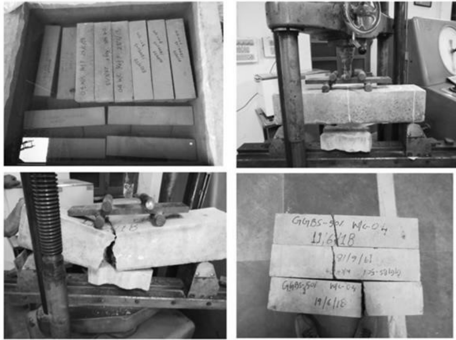
Figure 3.12 Curing and testing of FS
