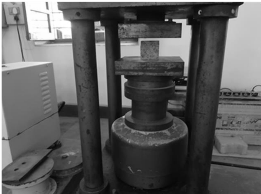
Figure 3.6 Compressive strength of mortar testing machine (UTM)
