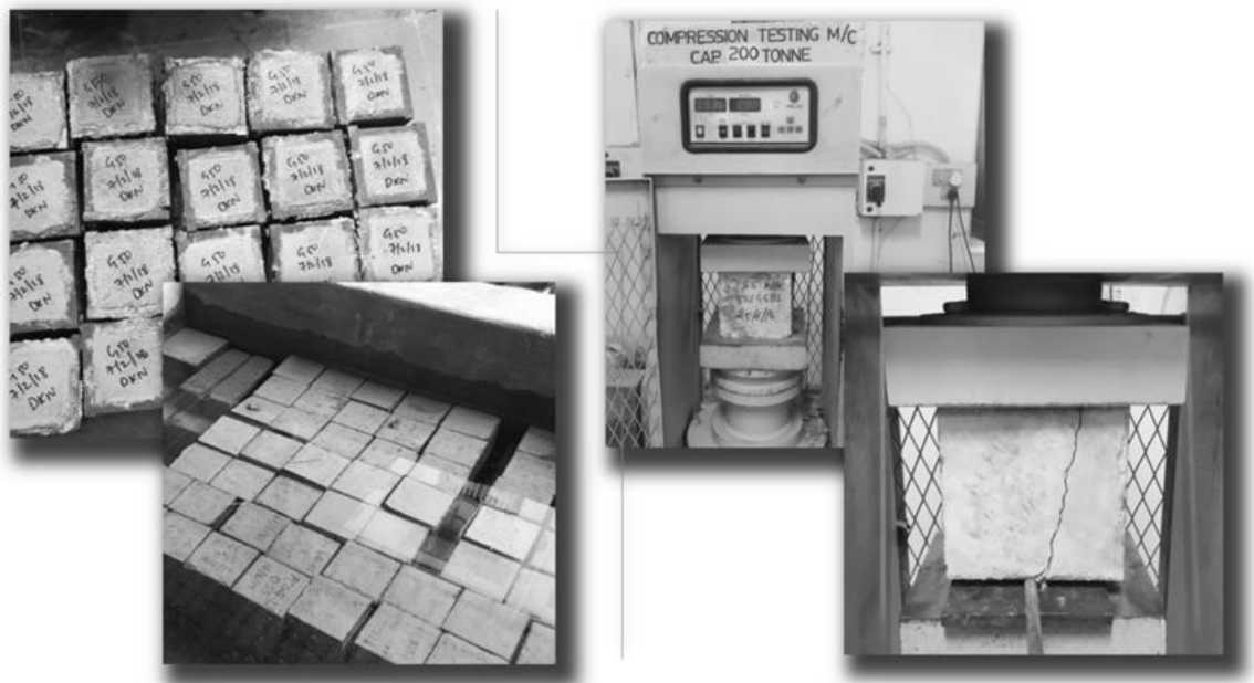
Figure 3.11 150 mm cube casting demolding and testing
