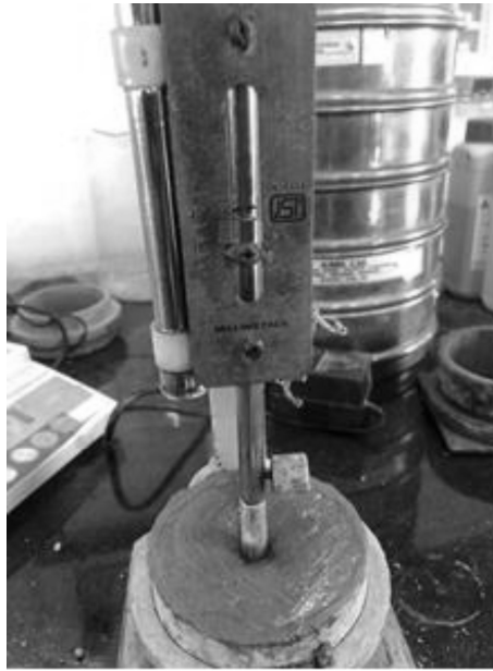
Figure 3.2 Vicat apparatus for setting time and standard consistency
