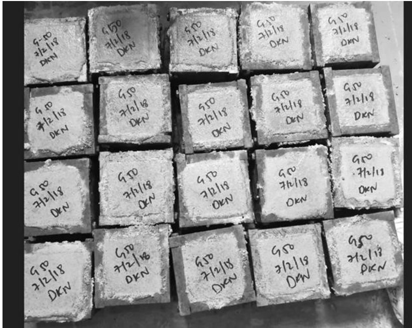
Figure 3.5 Casting of mortar cube
