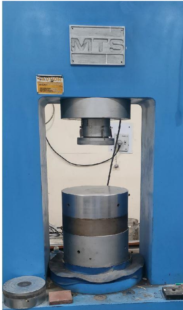
Figure 4.1. Material Testing System (MTS) facility used for coal testing at IIT (BHU), Varanasi
