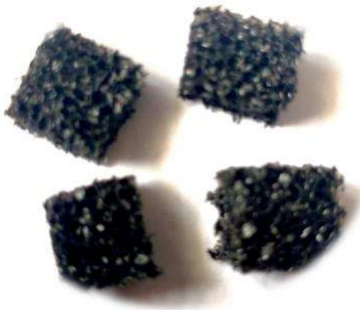
Figure 4.1. Low density polyethylene used as packing media in packed bed bioreactor.
