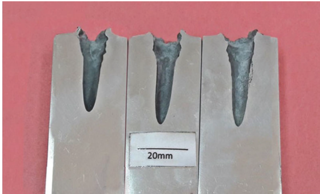
Fig 4.9: Half section views of the (i) ST (ii) LT and (iii) L direction impacted craters
