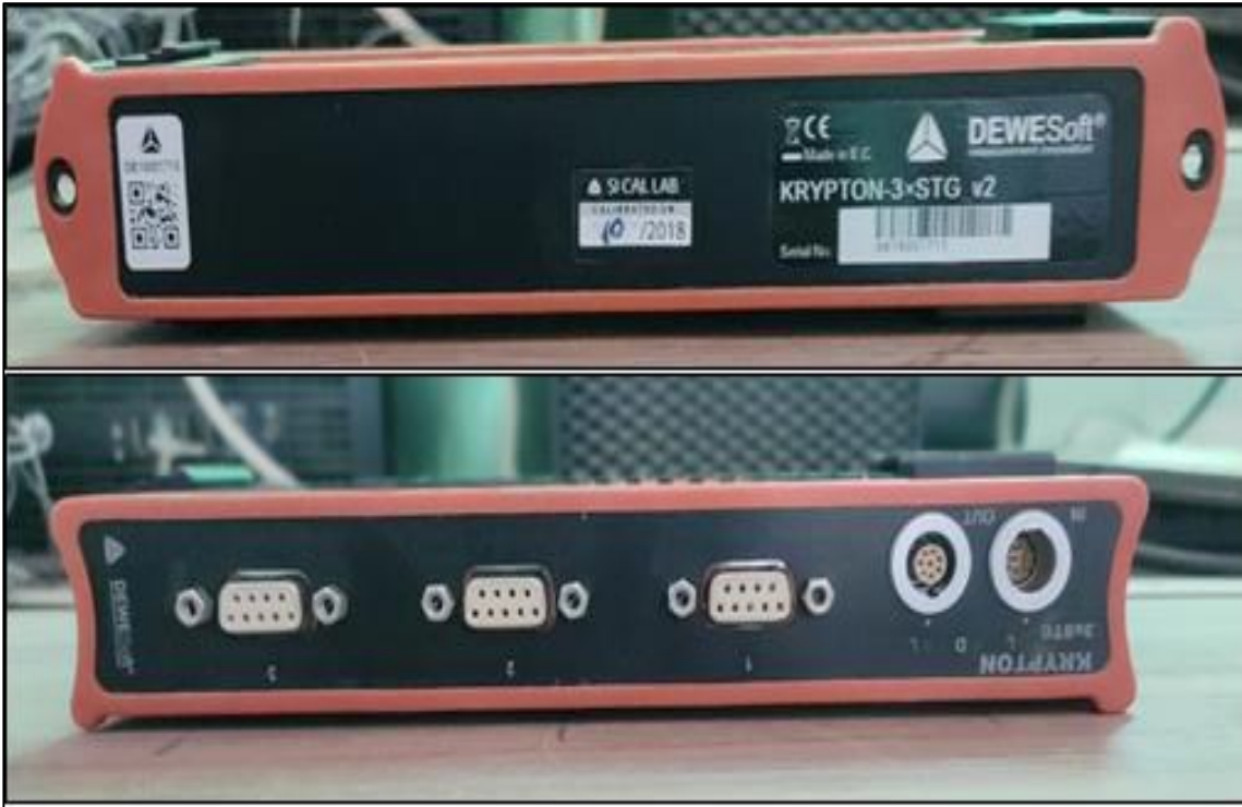
Fig. 5.13 Krypton-3-STG Data acquisition system
