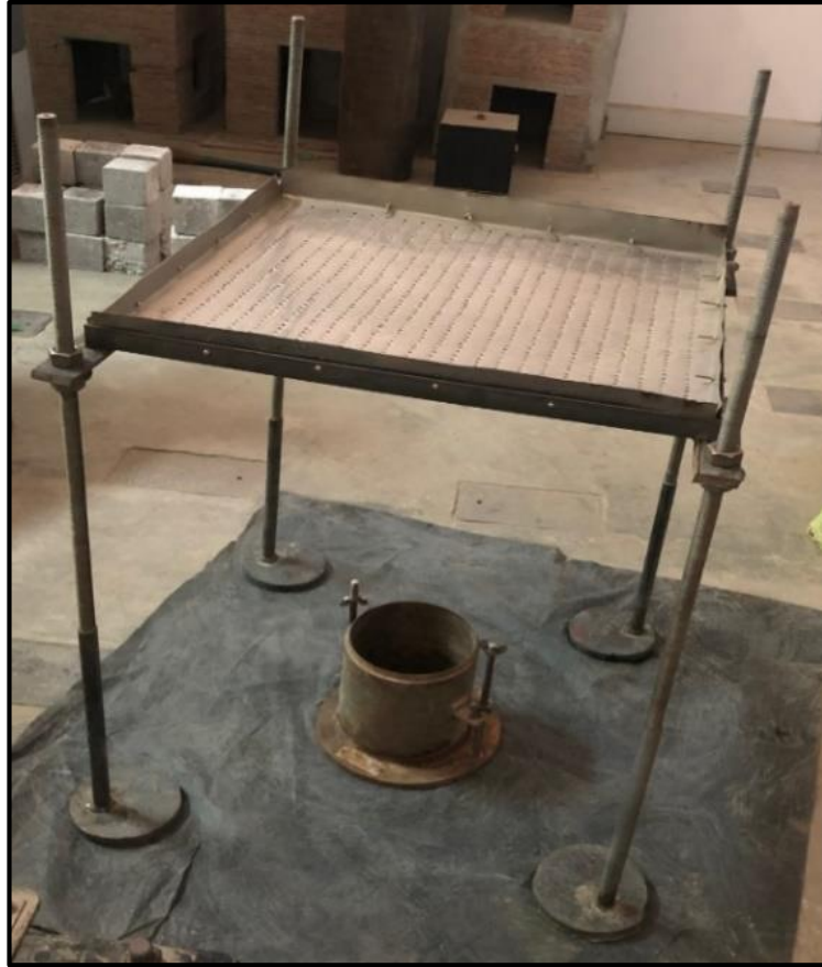
Fig. 5.11 Adjustable sieve arrangement for rainfall technique
