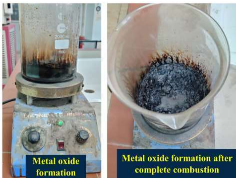
Figure 3.6: Experimental set-up used in the laboratory to synthesize metal oxides
