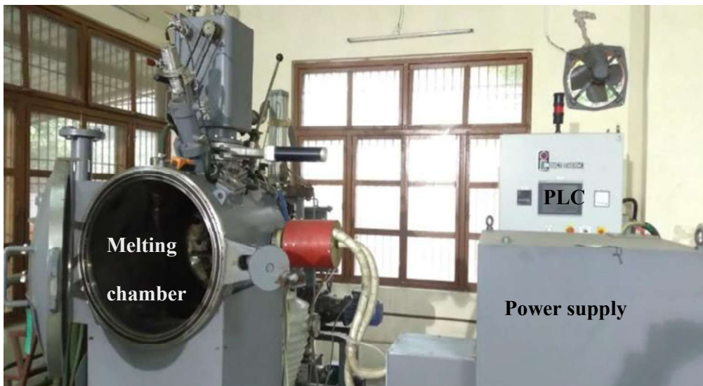
Fig. 8: Vacuum induction melting furnace setup.
