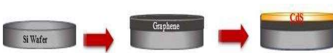
Figure 3.2. Address layer of cadmium sulfide sample grown on graphene
