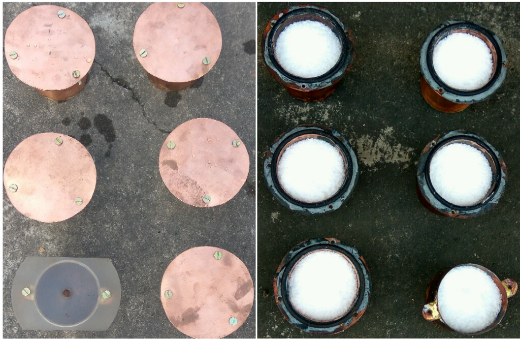
Fig. 3. Pictorial view of PCM loaded copper cylinders.
