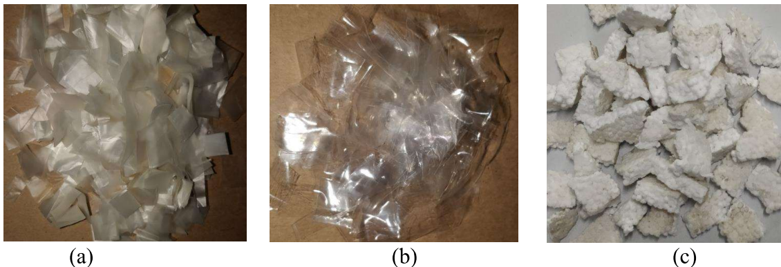
Figure 3.5 Pictorial view of feed materials (a) polyethylene, (b) polypropylene and (c) polystyrene
