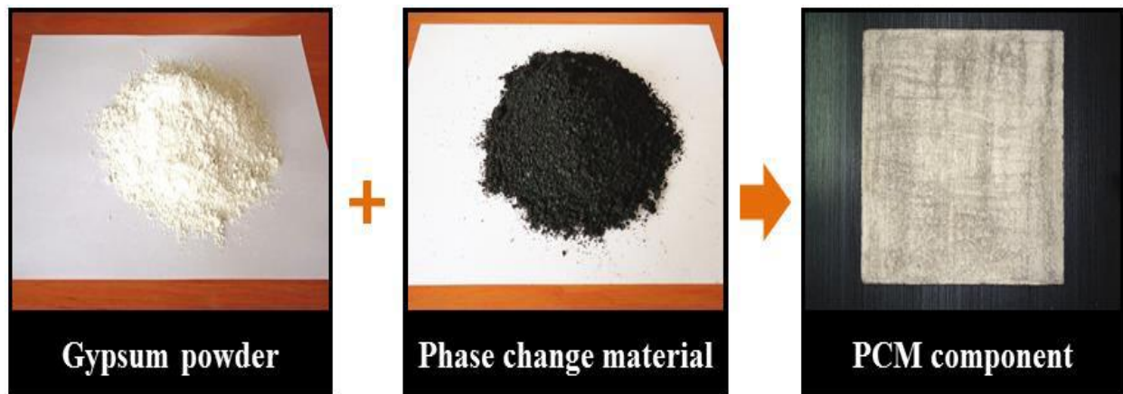
Figure 2.13 Gypsum powder, MPCM and prepared gypsum-MPCM panel (90)
