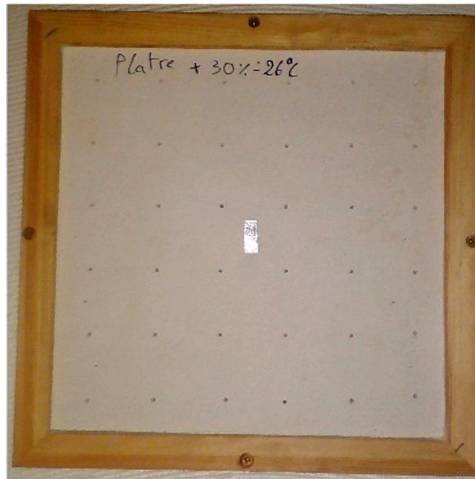
Figure 2.12 Perforated MPCM plasterboard with holes (89)
