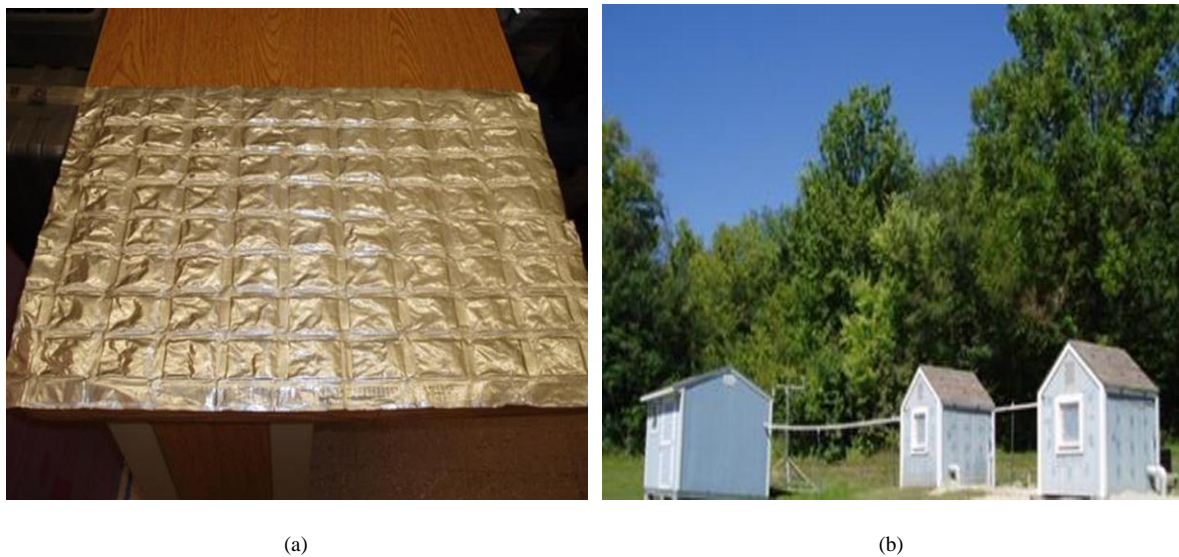
Figure 2.23 (a) PCM packed in aluminum foil sheet (b) Test houses developed for study (105)
