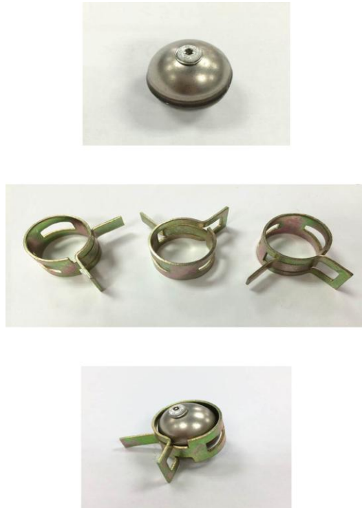
Figure 2.34 HSB without metal clamp, metal clamp and HSB with metal clamp (From top to bottom) (114)
