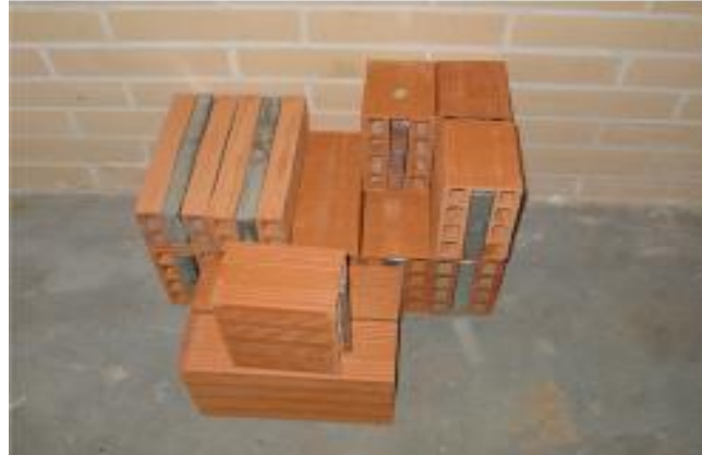
Figure 2.18 Bricks with PCM macrocapsules (101)
