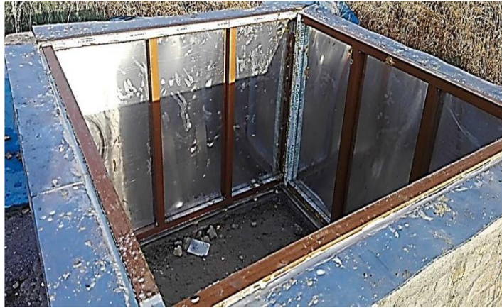
Figure 2.26 Test room with PCM encapsulation (108)
