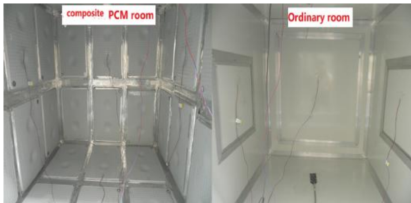
Figure 2.19 Inside view of composite PCM room and ordinary room (102)
