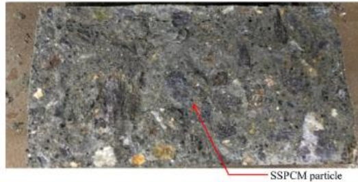
Figure 2.66 (a) Shape stabilized PCM (b) Concrete loaded with shape stabilized PCM (252)
