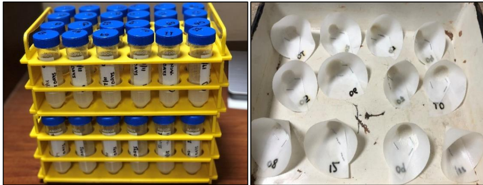
Fig. 6.1 (a) Falcon tubes containing EICP solution (b) Filter papers containing calcite precipitate
