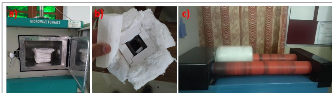
Figure 3.3 a) Microwave sintering furnace, b) heating space for sample and c) roller mixer
