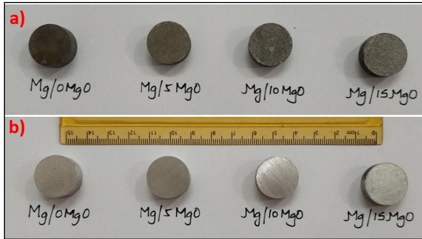
Figure 3.8 Sintered samples a) just after removing aluminium foil and b) after coarse polishing
