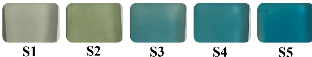
Fig. 4.2. Images of optically polished glass samples prepared for optical analysis are shown, where sample S1 has dimensions of 20.35 mm in length, 17.68 mm in breadth, and 7.96 mm in width; S2 measures 23.91 mm in length, 22.01 mm in breadth, and 8.10 mm in width; S3 has dimensions of 20.51 mm in length, 20.26 mm in breadth, and 8.01 mm in width; S4 measures 26.24 mm in length, 26.05 mm in breadth, and 8.06 mm in width; and S5 has dimensions of 18.50 mm in length, 17.17 mm in breadth, and 8.02 mm in width.
