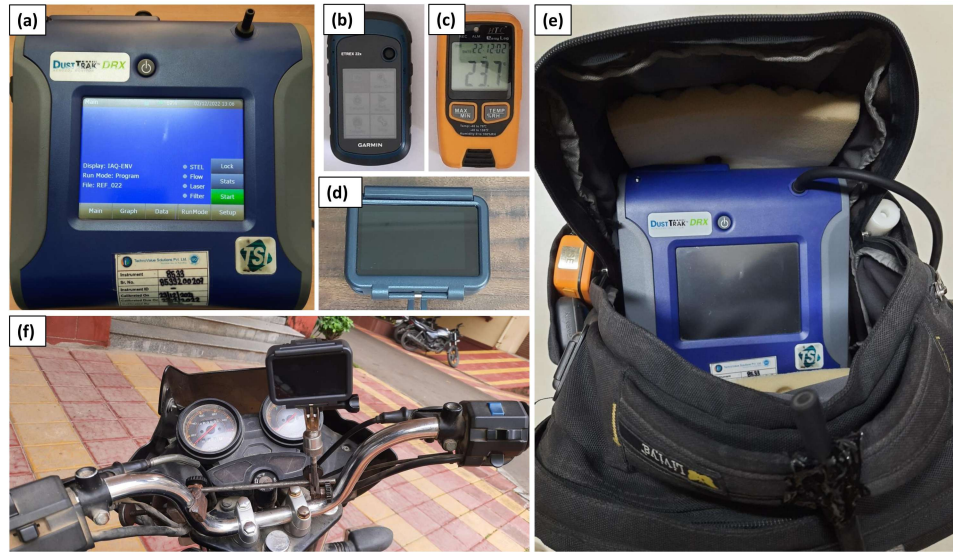
Fig. 3.3 Instrumentation setup: (a) DustTrak aerosol monitor for collecting PM concentration data; (b) Garmin device for GPS coordinates; (c) HTC data logger for RH and AT logging; (d) an action video camera (e) backpack with aerosol monitor, GPS receiver, and RH & AT data logger; (f) motorcycle fitted with action camera.
