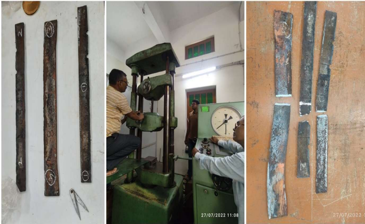
Figure 4.5: Lab-tested steel samples before, during and after the test
