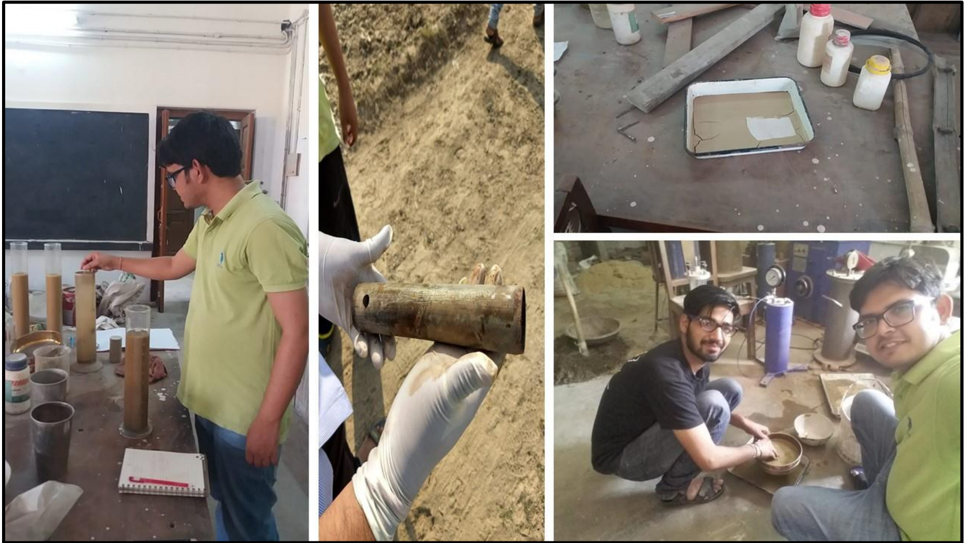
Figure 7.10 Soil texture analysis in the lab using Hydrometer test.
