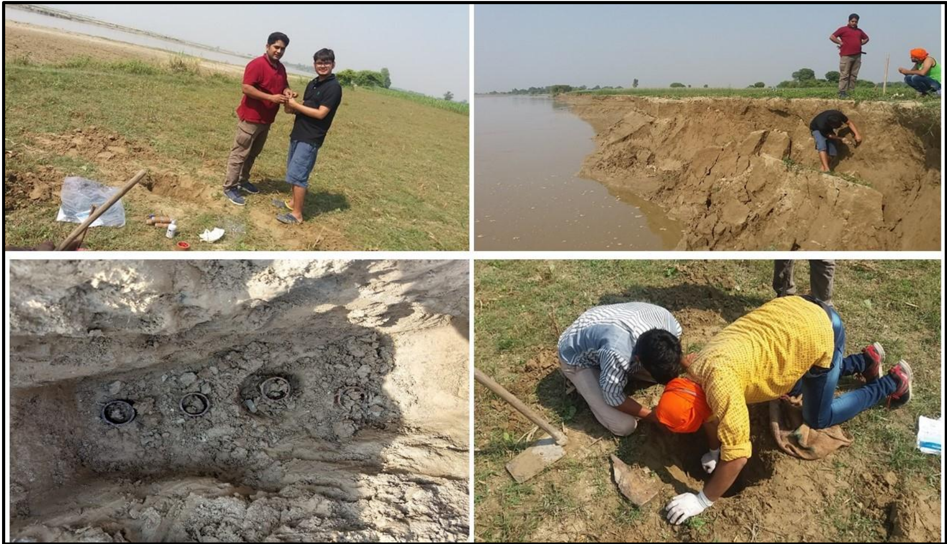
Figure 7.9 Soil sample collection using Shelby tube sampler in the field
