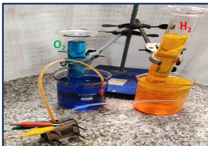
Figure 2.15 Photograph of indigenously designed electrolyzer setup showing production of \text{H}_2 and \text{O}_2 .
