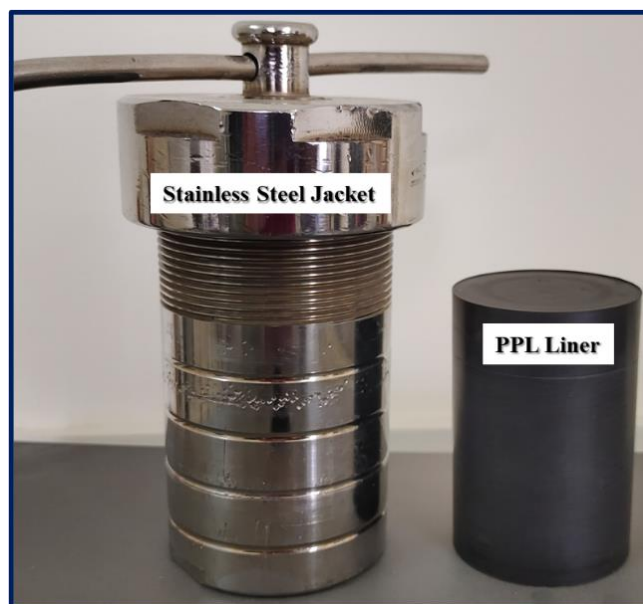
Figure 2.1 Photograph of the used hydrothermal cell
