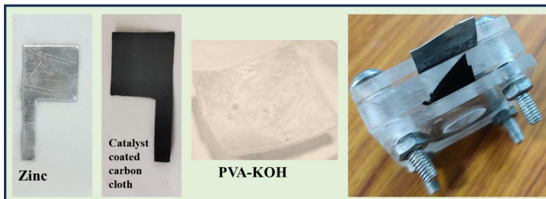
Figure 2.16 Different components and assembled Zinc-air battery.
