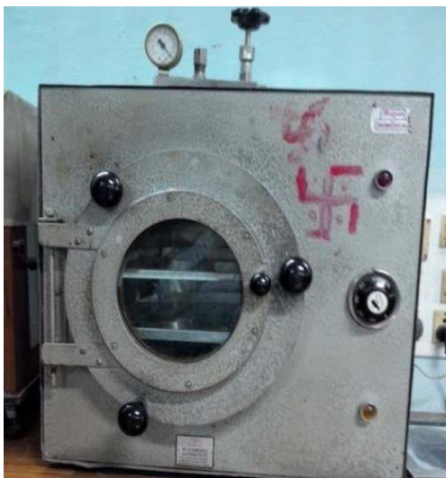
Fig. 2.19 Conventional box oven used for drying process
