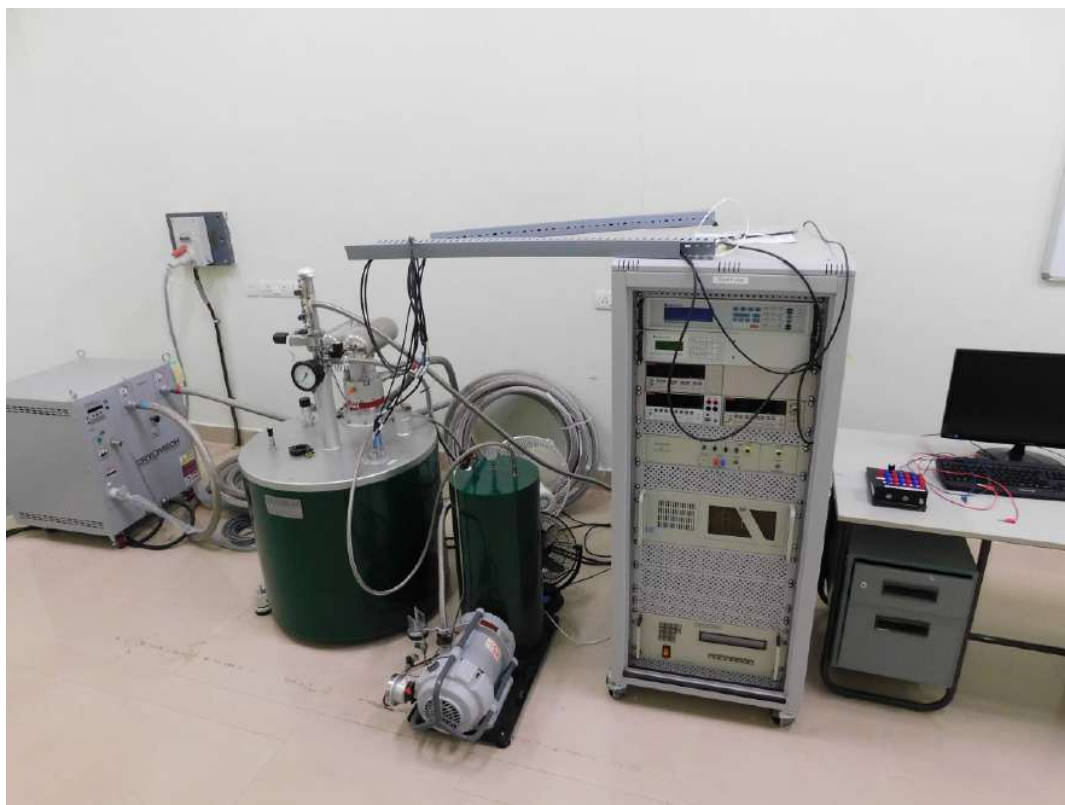
Figure 2.9: 15 T ppms machine for magnetotransport studies
