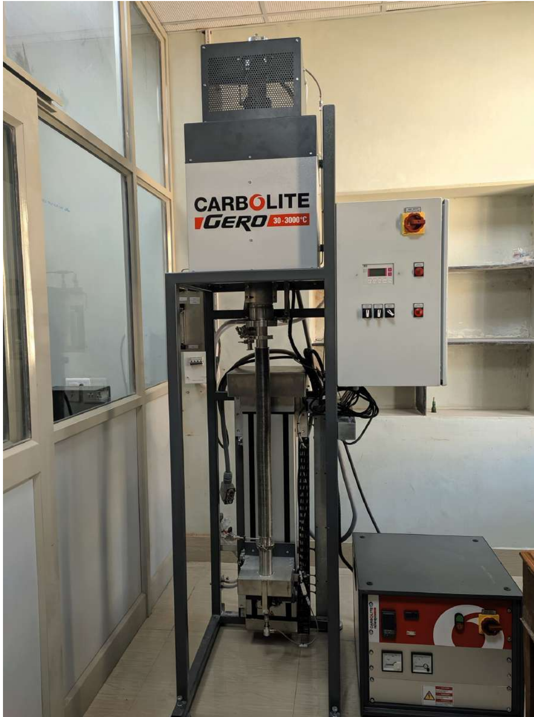
Figure 2.4: The Bridgman single crystal growth furnace. (Photograph taken from our laboratory)
