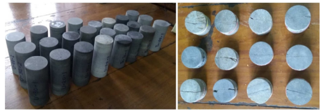
Fig. 4. F-T conditioned rock specimens NX size rock specimens for (a) UCS and (b) BTS.
