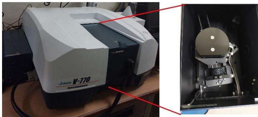
Fig. 2.9 UV-Vis spectrophotometer (Jasco V-770) equipped with an integrating sphere setup.
