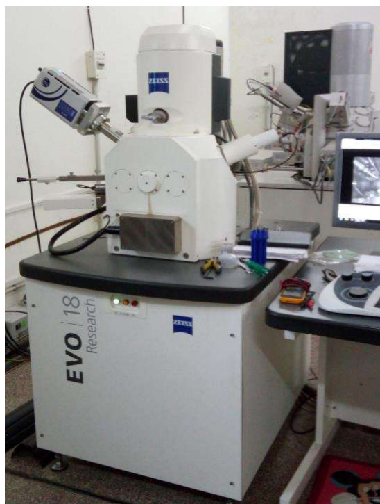
Fig. 2.5 SEM- EDS set up.
