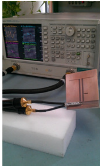
Figure 6.19: Measurement setup for S_{11} measurement
