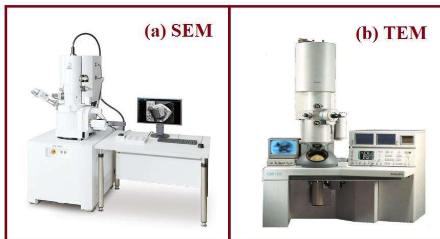
Fig. 2.5 Instrument setup of (a) Scanning Electron Microscope (SEM) and (b) Transmitted Electron Microscope (TEM).
