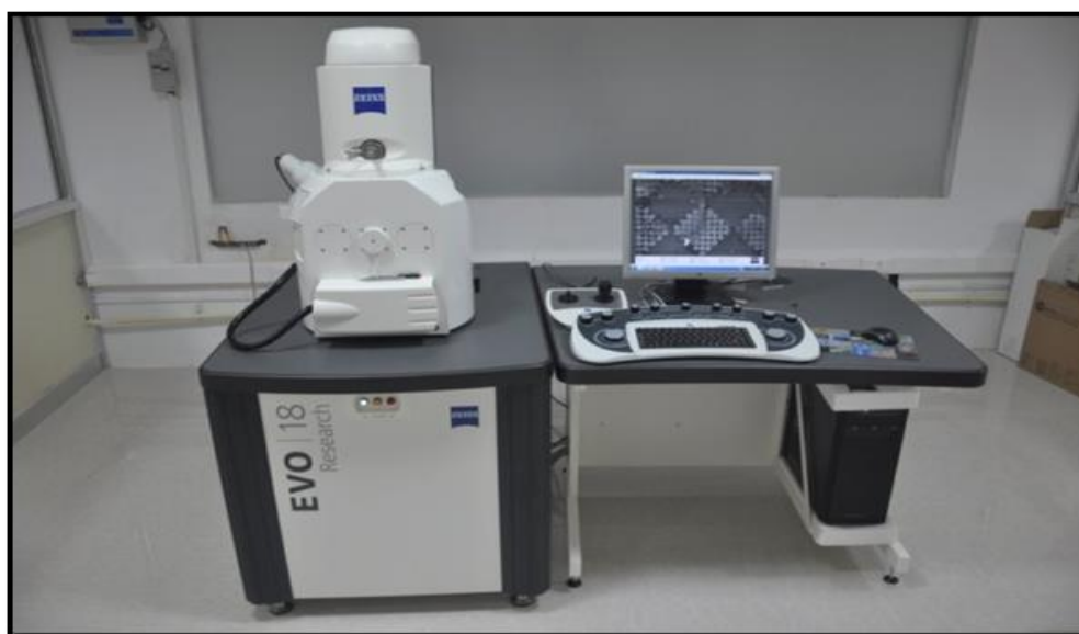
Fig. 2.5. Scanning Electron microscopy (SEM, ZEISS model, EVO18 Germany) and EDX Analysis instrument (Oxford instrument; USA)
