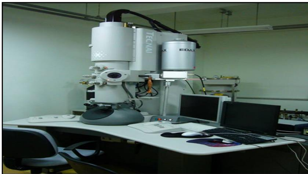
Fig.2.6. Transmission Electron Microscope (TEM, FEI TECANI G 2 20 TWIN, USA) used to determine particle structure.
